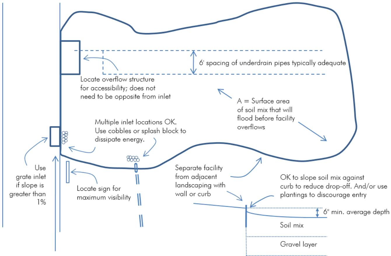
Note: Call out elevations of curb, pavement, inlet, top of soil layer (TSL), bottom of soil layer (BSL), and bottom of gravel layer (BGL) at all inlets and outlets and at key points along edge of facility.
