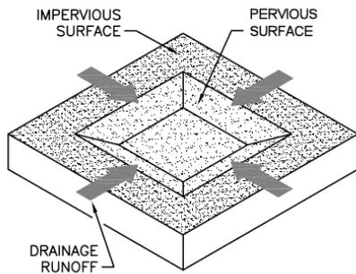
**Figure 4-2. Self-retaining areas** are designed to retain the first one inch of rainfall without producing any runoff. During intense storms, runoff may drain off-site, to the storm drain system, or to LID facilities.
